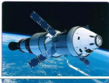
Crew module This is the only part of the Orion spacecraft that will return to Earth, using a parachute to splash down in the ocean.
